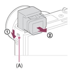
• If you slide the Viewfinder pop-up switch when the camera is off, the camera will turn on.
