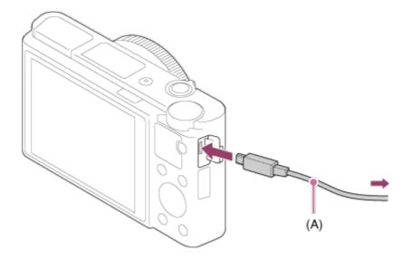
• If you connect the product to your computer using the micro USB cable when [USB Power Supply] is set to [On], power is supplied from your computer. (Default setting: [On])
